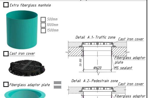
\*H-depth of the inlet connection (in standard equipment H up to 1000 mm. H take a multiple of 50mm.
